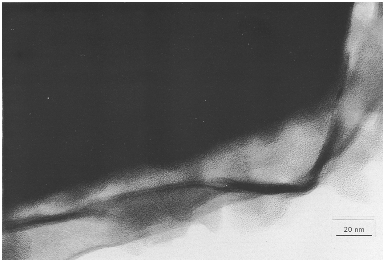
Figure 2 High-resolution transmission electron micrograph of the unfired (\text{C}_6\text{H}_{13}\text{NH}_3)\text{Nb}_3\text{O}_8/\text{PAN} composite (1b).
